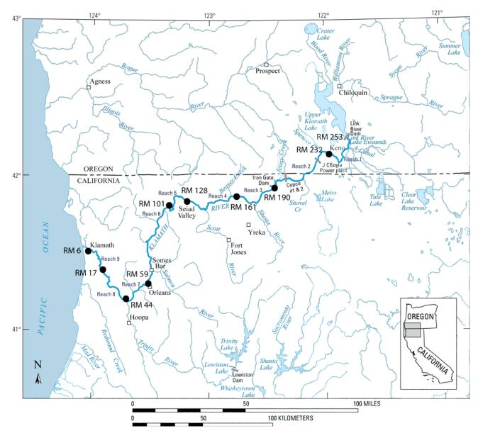
**Figure 1.** Map of the Klamath River showing the study area from Link River Dam to the Pacific Ocean. Points (•) mark locations with observed temperature data (RM = river mile) used for calibration and for separating the river into nine model reaches.
