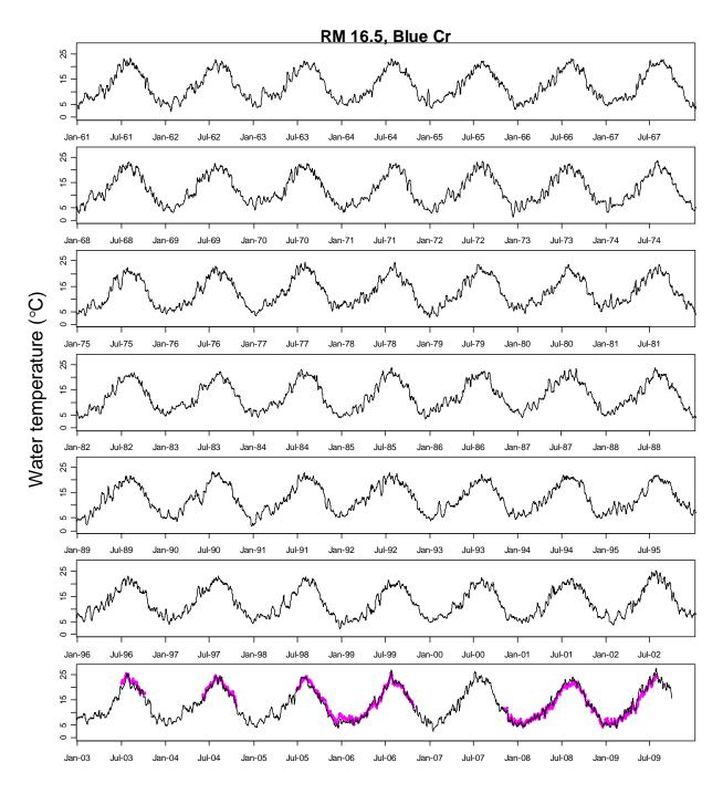
**Figure A8.** Time series of predicted (solid line) and observed water temperature (o) of the Klamath River at river mile (RM) 16.5.
