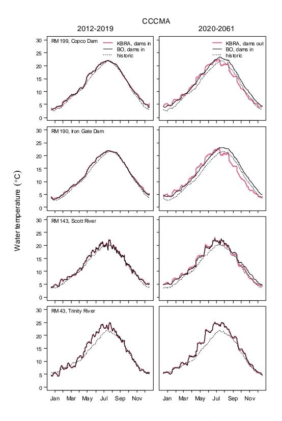
**Figure A12**. Mean temperature by Julian day for the KBRA dams in period (left panels) and dams out period (right panels) at four locations on the Klamath River for the CCCMA General Circulation Model (GCM). The historical simulation is shown as a baseline and represents mean temperatures by Julian day for 1961–2009.
