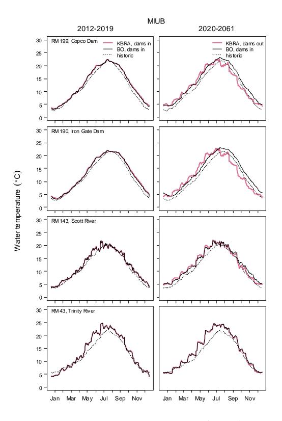
**Figure A13**. Mean temperature by Julian day for the KBRA dams in period (left panels) and dams out period (right panels) at four locations on the Klamath River for the MIUB General Circulation Model (GCM). The historical simulation is shown as a baseline and represents mean temperatures by Julian day for 1961–2009.
