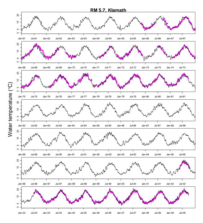
**Figure A9.** Time series of predicted (solid line) and observed water temperature (o) of the Klamath River at river mile (RM) 5.7.
