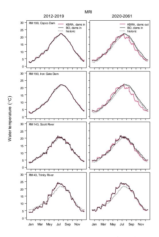
**Figure A10**. Mean temperature by Julian day for the KBRA dams in period (left panels) and dams out period (right panels) at four locations on the Klamath River for the MRI General Circulation Model (GCM). The historical simulation is shown as a baseline and represents mean temperatures by Julian day for 1961-2009.
