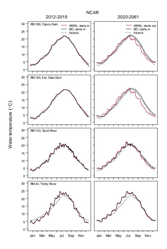
**Figure A11**. Mean temperature by Julian day for the KBRA dams in period (left panels) and dams out period (right panels) at four locations on the Klamath River for the NCAR General Circulation Model (GCM). The historical simulation is shown as a baseline and represents mean temperatures by Julian day for 1961-2009.
