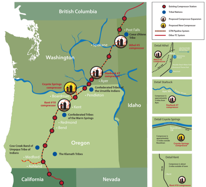
Map of GTN Pipeline and Compressor Stations
